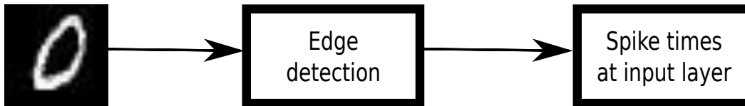
Figure 5: A block diagram of the encoding model that processes MNIST images to produce patterns of spike times
